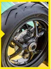
Pirelli's famous lightning element tread pattern not only disperses water, it works with the connecting elements to minimise warm-up times. The overall void/fill ratio of the tyre is just six per cent.
